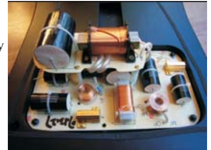
A passive crossover: coils, capacitors and resistors
